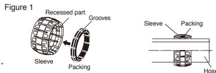
※ Fit the sleeve with the packing attached. If the packing comes off from the sleeve or becomes twisted, refit the packing with its outer circumferential grooves facing outwards to the recessed part of the sleeve as shown in figure .
