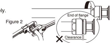
4. Fasten the hose to the pipe using a commercially available sanitary clamp. Mount the hose onto the pipe, making sure that the hose is not twisted.
